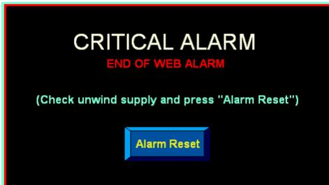
The critical alarm includes: Out of Labels, Out of Ribbon, and End of Web. Label and ribbon alarms come from the printer and you should consult the printer manual as to how the signals are set. The End of Web signal comes from a sensor mounted to look for the label supply to end before entering the printer. When a critical alarm occurs, the applicator will stop applying labels.
