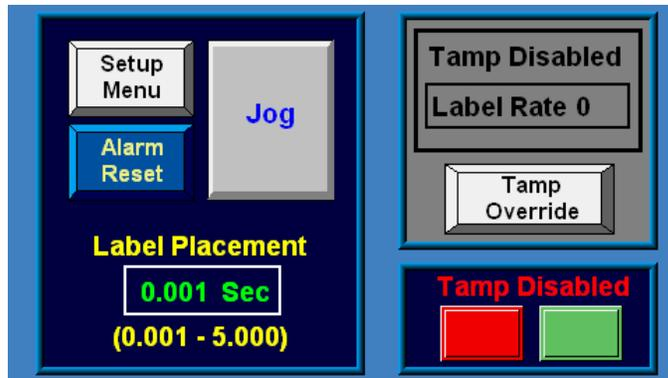
The left side of the screen will remain the same. There will always be jog, alarm reset keys and access to label placement time adjustments. Label Placement is the time from when the product detect sensor turns on until the labeling sequence starts. This is the tool used to place the label in the right position on the product.
