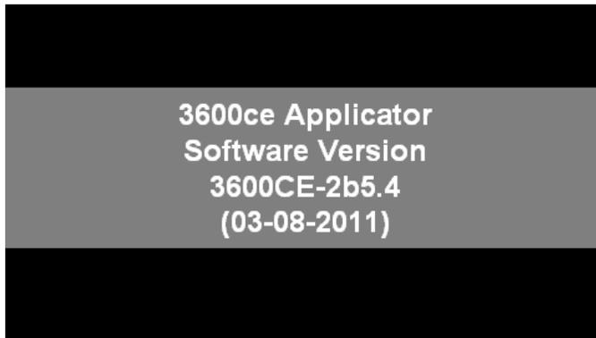
On power-up, the display will scroll the software version screen for 10 or 45 seconds. Zebra equipped printer applicators take 45 seconds to start up. Sato equipped printer applicators take 10 seconds to start up. This startup time allows for the print engines to go through their diagnostics.
