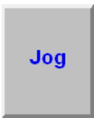
The Jog key is used to jog a label onto the pad when the tamp is disabled or to jog a labeling sequence while the tamp is enabled.
