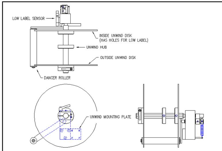
Figure 1 (Unwind Assembly)
