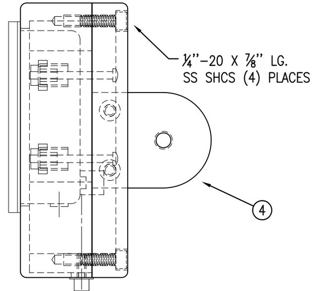
DISPLAY ASSEMBLY CAN ALSO BE MOUNTED FROM THIS SIDE BY REMOVING (4) 1/4"-20 X 3/4" SHCS & THEN ROTATING DISPLAY BACK SHELL 180° (ITEM 3)
