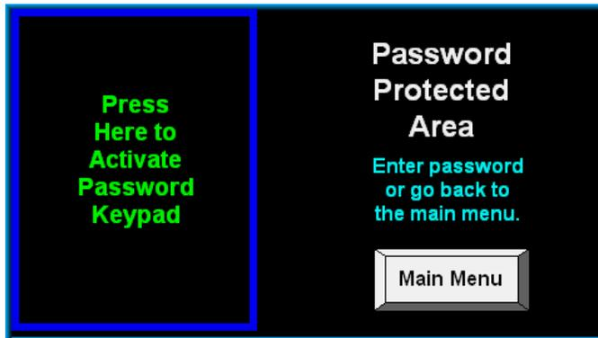
Once the operator has disabled the tamp and presses the configuration menu key again this screen will pop up notifying the operator that the area is password protected. Here the operator can chose to go back to the main menu or continue with password entry by touching within the box to the left to invoke the keypad.
