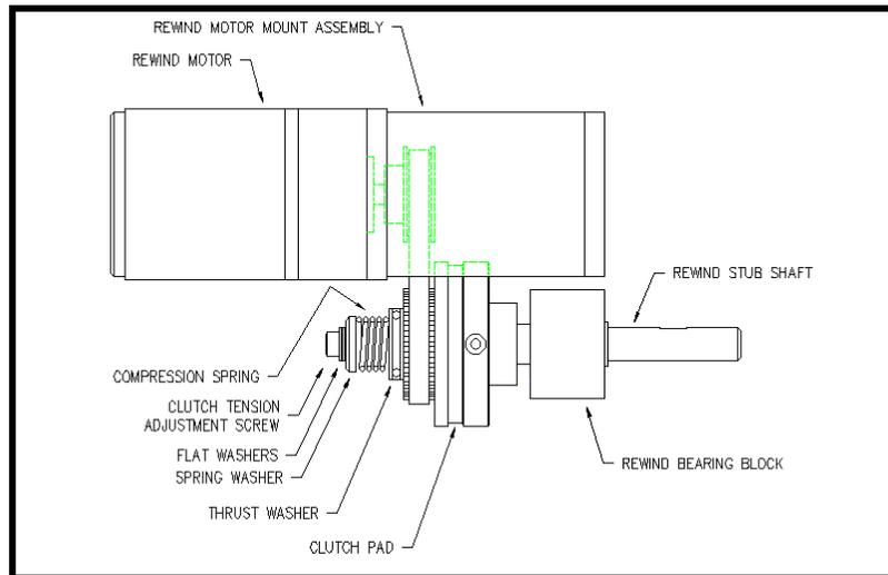
Figure 18 (rewind/clutch assembly)
