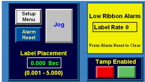
The warning alarm will activate on the following conditions: Low Label and Low Ribbon. The low label signal comes from a photoelectric sensor mounted on the side of the unwind bearing block. This sensor can be adjusted to turn on at different roll diameters. The low ribbon signal comes from the printer (Consult the printer manual). On a warning alarm the applicator will continue to apply labels.
