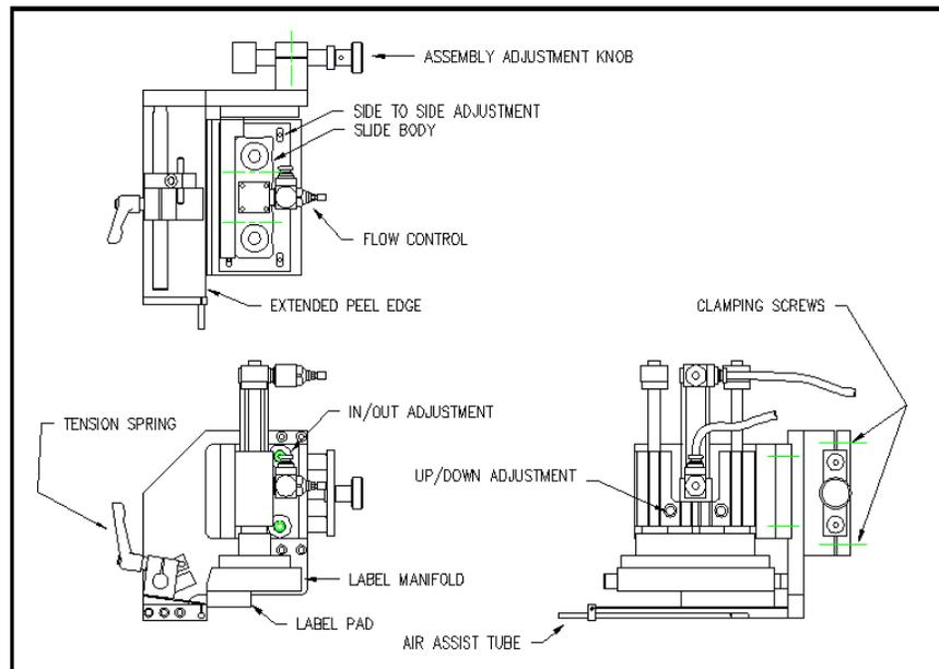
Figure 4 (Extended Peel Edge Assembly)
