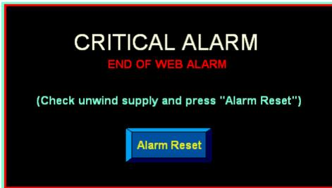
The critical alarm includes: Out of Labels, Out of Ribbon, and End of Web. Label and ribbon alarms come from the printer and you should consult the printer manual as to how the signals are set. The End of Web signal comes from a sensor mounted to look for the label supply to end before entering the printer. When a critical alarm occurs, the applicator will stop applying labels.
