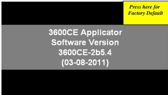
The ability to reset to factory defaults is useful when the applicator will not dispense labels due to a configuration problem. Resetting to factory defaults will bring all of the settings to something that works and adjustments can be made from there. The factory default screen can be accessed from the power-up software screen.
