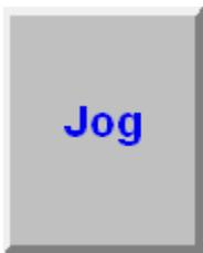
The Jog key is used to jog a label onto the pad when the tamp is disabled or to jog a labeling sequence while the tamp is enabled.
